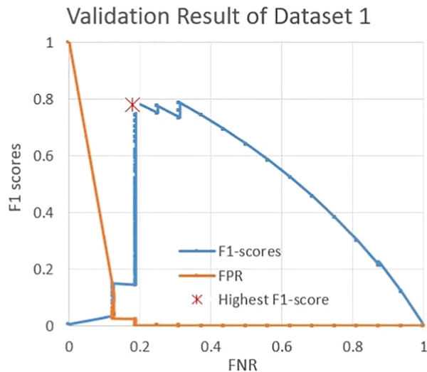
Fig. 5. Validation results of FN-Net for Dataset 1 at various FNR values. The best F1 scores (red crosses) are the commonly used points in threshold selection. However, any points in the graph are feasible solutions.
